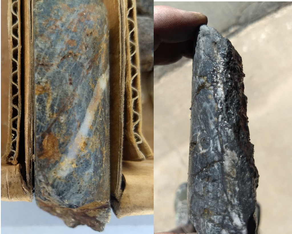
Figure 7-5 Photographs of selected core specimens within sampled intervals of high-grade gold (left T-701C, 47 ft; right, T-706C 240 ft)
