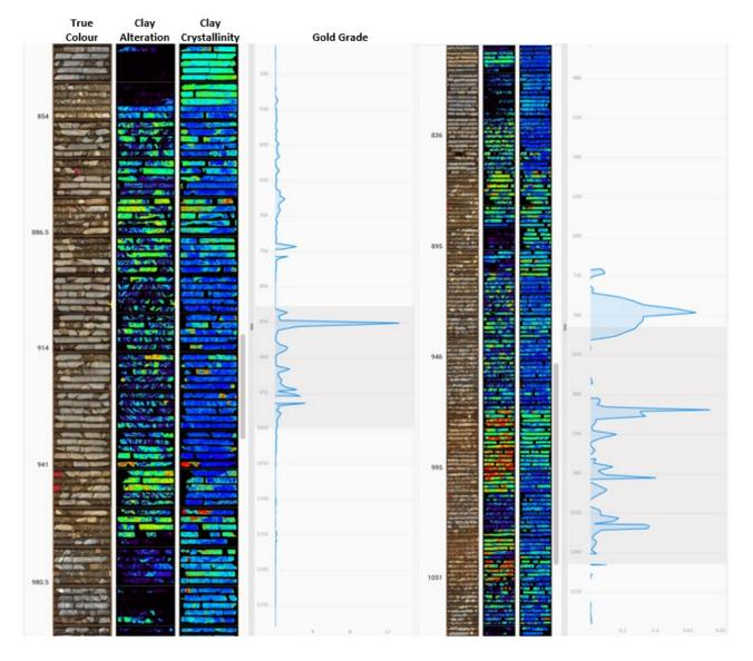
Figure 2: Hyperspectral Imaging – Drill holes T-1601 (Left) & T-1602 (Right)
